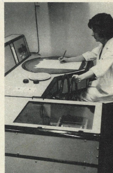
Two views of the two-mirror distribution photometer. Curves are plotted at the table by marking the position on the graph paper of the spot of light from the galvanometer sited on the wall above.
